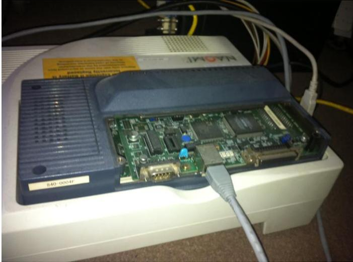
Insert the Network Security chip, make sure it's the right way round if you're not using a proper key holder.
